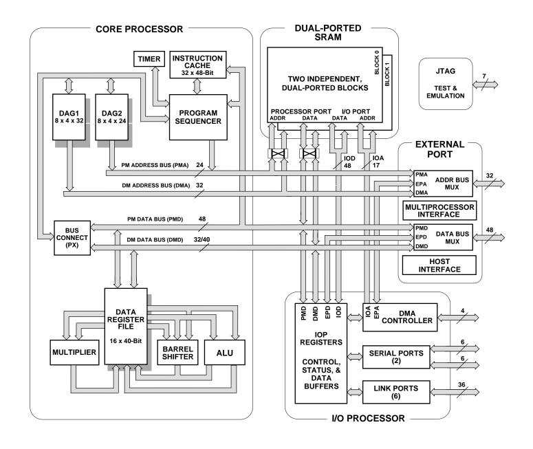
Figure 2. ADSP-21060 Architecture Block Diagram
