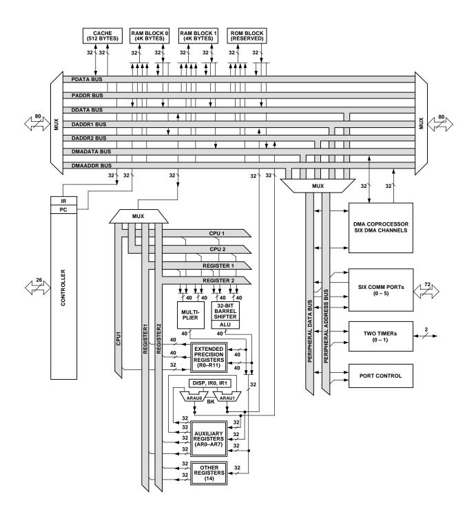
Figure 1. TMS320C40 Architecture Block Diagram
